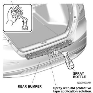
3. Remove the adhesive backing from the side of the rear bumper applique with the 3M mark.
