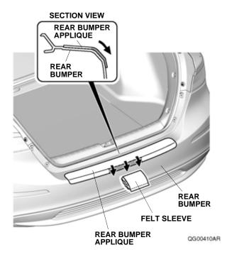
11. Repeat step 8 at the left and right sides of the lower section on the rear bumper applique.
