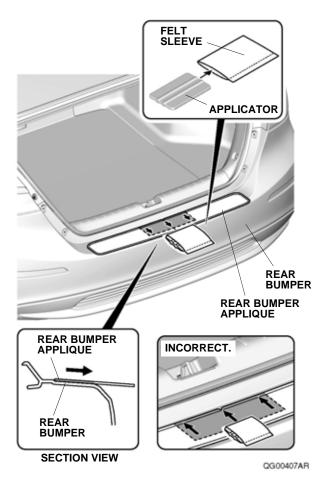
7. Starting from the front and working rearward, use the felt sleeve to smooth out the center of the upper section on the rear bumper applique. Move the felt sleeve in one direction only. If you see an air bubble, stop and gently peel up that section to work out the bubble. Work slowly, and keep pressure against the rear bumper applique.
