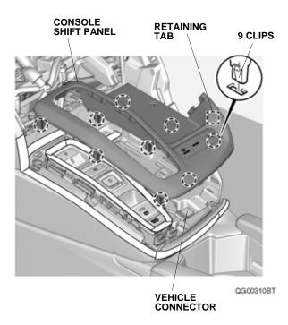
13. Remove the switch panel, and unplug the vehicle connectors.
