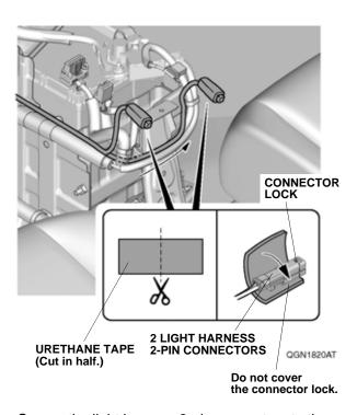
51. Secure the light harness 2-pin connectors to the vehicle harness with the two wire ties.
