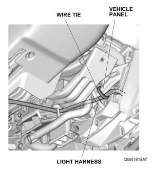
47. Install the relay and the clip to the light harness relay block.
