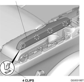
18. Remove the console rear panel, and unplug the vehicle connectors.
