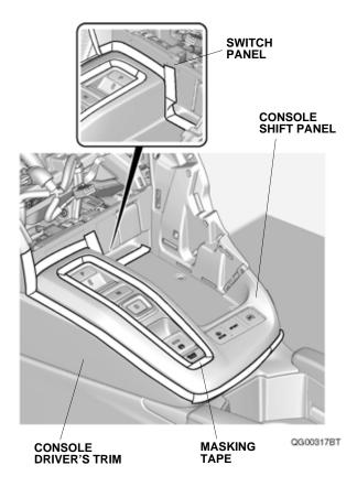
12. Remove the console shift panel, and unplug the vehicle connector.
