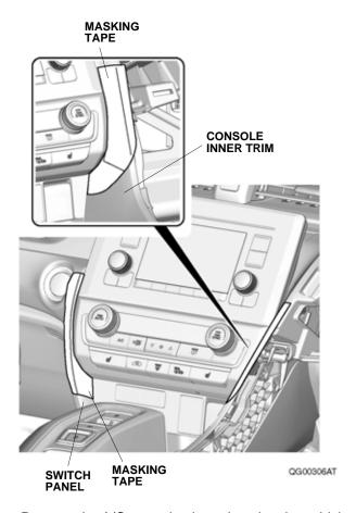
6. Remove the A/C control unit, and unplug the vehicle connector.
