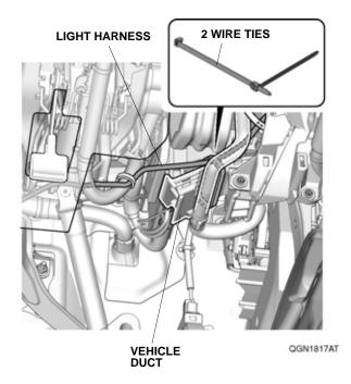
46. Secure the light harness to the vehicle panel with one wire tie.
