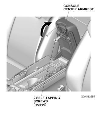
Install the new left console side armrest to the center console.
