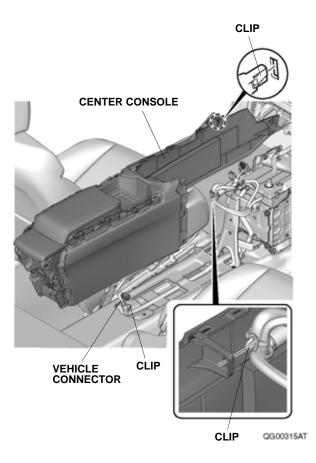
20. Remove the driver's dashboard lower cover, and unplug the vehicle connectors.
