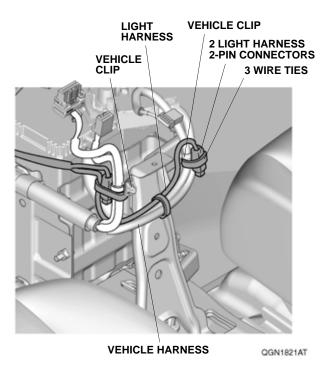
52. Secure the light harness to the vehicle harness with one wire tie.
