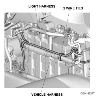
54. Plug the left and right light 2-pin connectors into the light harness 2-pin connectors, and install the center console.
