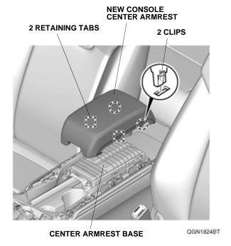
56. Open the console center armrest, and secure it with the two self-tapping screws.
