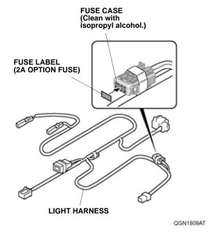
36. Apply the fuse label to the light harness fuse case.
