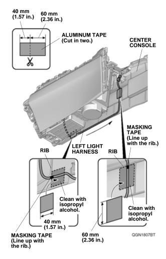
Using scissors, cut one piece of aluminum tape as shown. Secure the left light harness to the center console with two pieces of aluminum tape.
