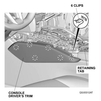
15. Remove the console panel, and unplug the vehicle connectors.
