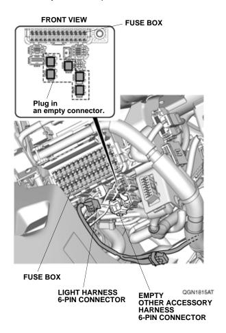
44. Secure the light harness to the vehicle harness with the three wire ties.
