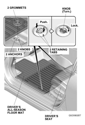
Place the grommets in the driver's all-season floor mat over the anchors. Push the grommets into the anchors to secure the retaining tabs, then turn the knobs 90° to secure the driver's all-season floor mat. 3. Install the passenger's all-season floor mat as shown.
