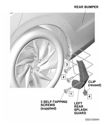
9. Turn the steering wheel fully clockwise, and repeat steps 2 through 8 to install the right splash guards.
