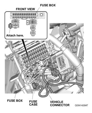
Route the door sill trim harness as shown. Secure it to the vehicle harness and bracket with the four wire ties.
