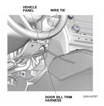
24. Route the door sill trim harness as shown. Secure the door sill trim harness to the vehicle harness with the four wire ties.
