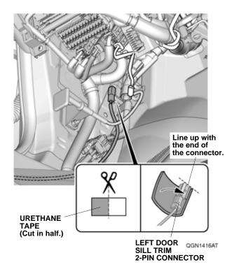
44. Plug the door sill trim harness 2-pin connector into the left door sill trim 2-pin connector.
