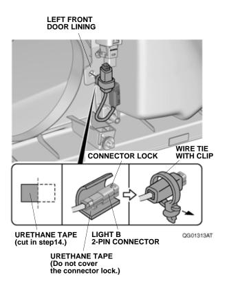
22. Plug the door lining illumination harness 2-pin connector into the light A 2-pin connector.
