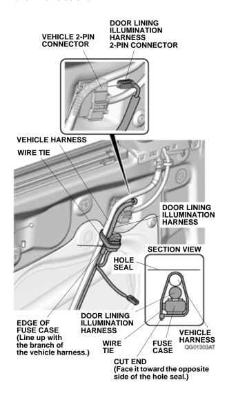
9. Secure the door lining illumination harness to the vehicle harness with two wire ties as shown.
