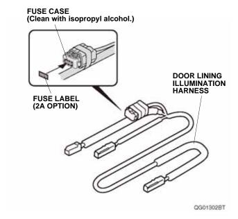
27. Attach the fuse label to the door lining illumination harness fuse case.
