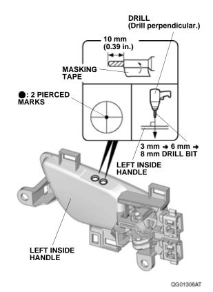
12. Using a file, remove any burrs from the holes.
