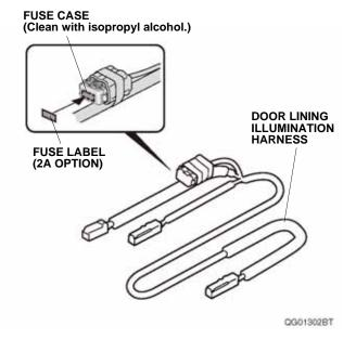
Attach the fuse label to the door lining illumination harness fuse case. 8. Plug the door lining illumination harness 2-pin connector into the vehicle 2-pin connector. Line up the edge of the fuse case on the door lining illumination harness with the branch of the vehicle harness, and secure it to the vehicle harness with one wire tie as shown.
