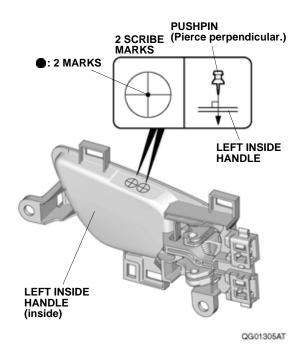
11. While wearing eye protection, drill the two pierced marks to 8 mm. First, drill with a 3 mm drill bit, then follow with a 6 mm drill bit, and finish with an 8 mm drill bit.
