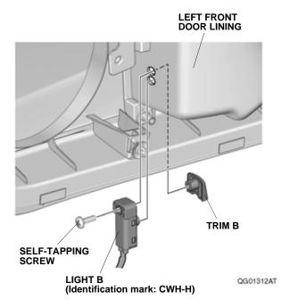
21. Using the other piece of urethane tape cut in step 14, wrap the light B connector, and secure the light B connector to the left front door lining with one wire tie with clip.
