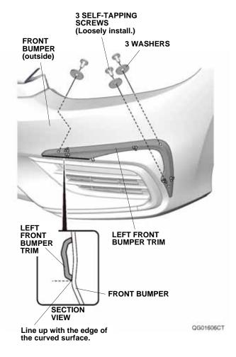
9. While applying light pressure against the left front bumper trim, carefully remove the adhesive backings as shown.
