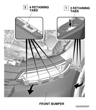
With the help of an assistant, remove the front bumper using a plastic trim tool, and unplug the vehicle connectors (if equipped). Place the front bumper on a blanket to prevent damage.
