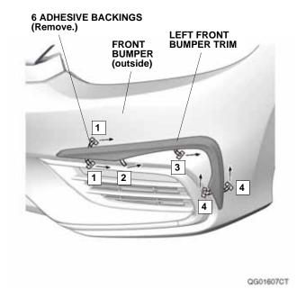
10. Using the rubber roller, apply firm pressure while rolling, especially at the ends, to set the adhesive.
