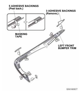
8. Line up the left front bumper trim with the front bumper as shown. Loosely install the left front bumper trim to the front bumper with three self-tapping screws and three washers.
