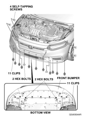
• With the help of an assistant, release the seven retaining tabs on each side.
