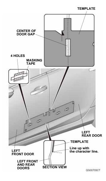
Using an alcohol wipe, thoroughly clean the left front door where the left front body side molding will attach.
