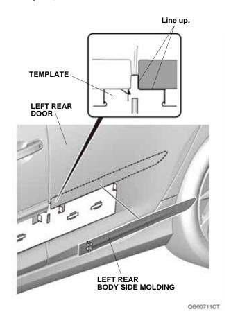
11. While applying light pressure against the left rear body side molding, carefully remove the taped adhesive backings.
