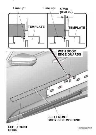
7. While applying light pressure against the left front body side molding, carefully remove the taped adhesive backings.
