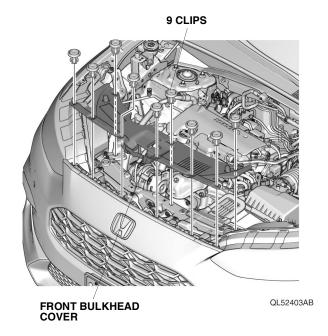
4. Remove the self-tapping screws and clips.
