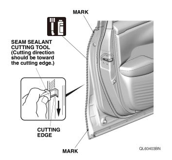
5. Temporarily install the left rear door edge guard.
