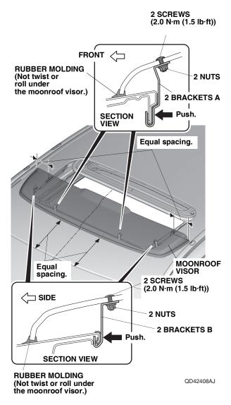
13. Tighten two screws and two nuts on the front of the vehicle first, then tighten two screws and two nuts on each side. Tighten while applying pressure so that there is no gap between the roof panel and the brackets A and B. Torque the screws to 2.0 N·m (1.5 lb·ft).
