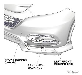
Using a rubber roller, apply firm pressure against the left front bumper trim and roll from one end to the other.
