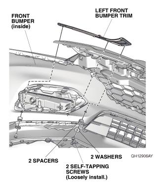
While applying light pressure against the left front bumper trim, carefully remove the adhesive backings.
