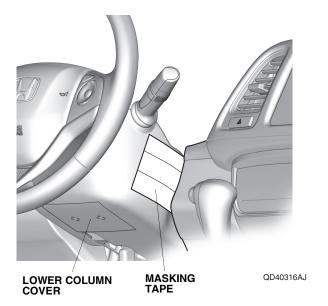
Pull away the door opening seal. Remove the driver's dashboard lower cover, and unplug the vehicle connectors.
