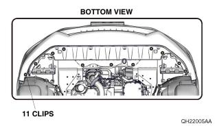
Remove the two self-tapping screws and four clips on each side.
