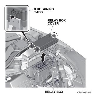
55. Using isopropyl alcohol on a shop towel, clean the relay box cover.
