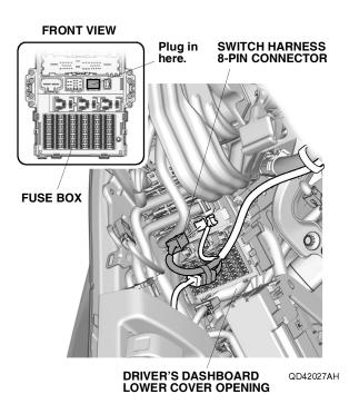
46. Secure the switch harness to the vehicle harness with one wire tie.
