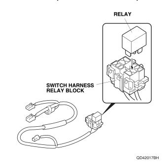
36. Plug the switch harness 1-pin connector into the vehicle 1-pin connector.
