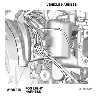
22. Line up the branch of fog light harness with the branch of vehicle harness, and secure the fog light harness to the vehicle harness with three wire ties.
