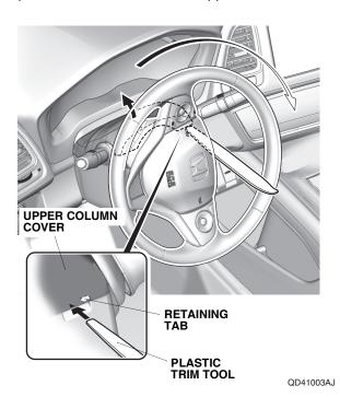
4. Turn the steering wheel 180° counterclockwise. Using a plastic trim tool, release the upper column cover.
