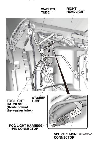
18. Plug the vehicle 1-pin connector into the fog light harness 1-pin connector.
