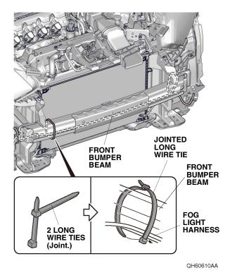
32. Using isopropyl alcohol on a shop towel, thoroughly clean the front bumper beam where the aluminum tape will attach.
