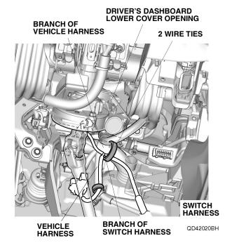
39. Secure the switch harness to the vehicle harness with three wire ties.
