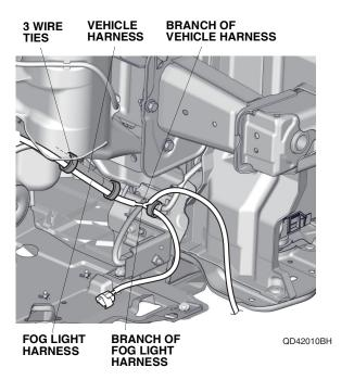
23. Secure the fog light harness clip to the hole in the vehicle frame as shown.
