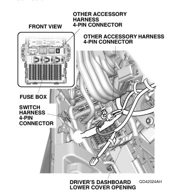
If the vehicle is equipped with another accessory harness 8-pin connector, go to step 44; otherwise, continue with step 43.
