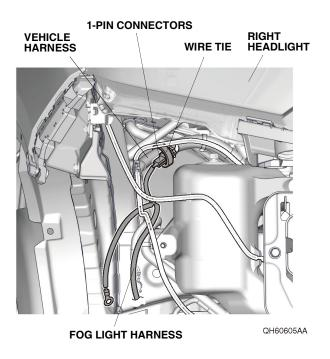
20. Route the fog light harness as shown. Install the fog light harness ground terminal to the vehicle panel with one ground bolt.
