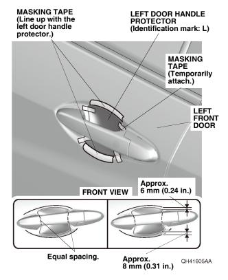
Attach masking tape to the left front door above and below the left door handle protector as shown.
