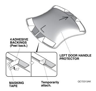
5. Line up the left door handle protector with the masking tape attached in step 3, and attach it to the left front door as shown.
