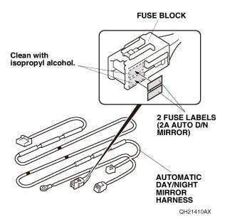
23. Attach the two fuse labels (2A AUTO D/N MIRROR) to the fuse block on the automatic day/night mirror harness.
