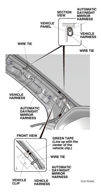
37. Secure the automatic day/night mirror harness to the vehicle harness with one wire tie.
