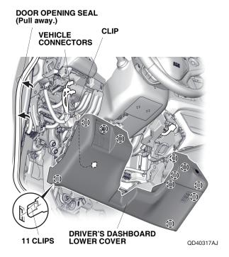
17. Pull away the door opening seal, and remove the driver's front door sill trim.
