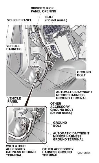
46. Secure the automatic day/night mirror harness to the vehicle harness with one wire tie.
