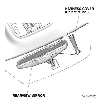
3. Loosen the TORX screw. Remove the rearview mirror, and unplug the vehicle connector. Go to step 5.
