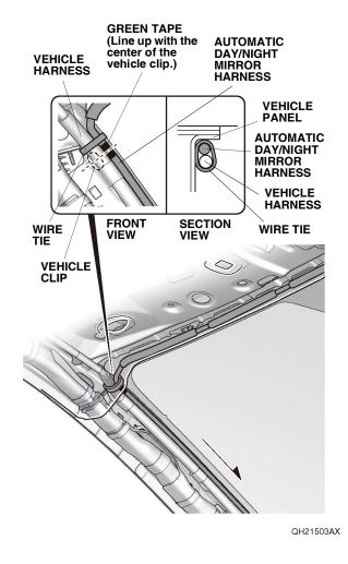
36. Line up the green tape on the automatic day/night mirror harness with the vehicle clip, and secure the automatic day/night mirror harness to the vehicle harness with one wire tie.
