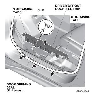
18. Pull away the door opening seal, and remove the driver's kick panel.
