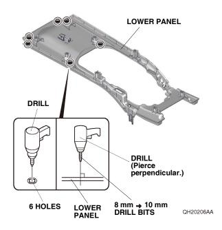
31. Install the left and right light, to the lower panel as shown.
