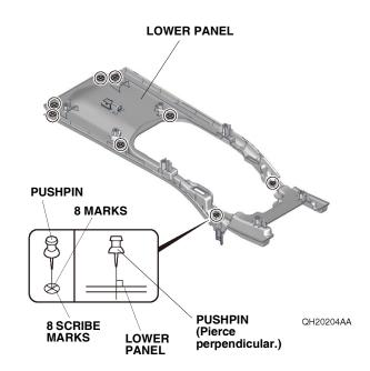
29. While wearing eye protection, drill the eight pierced marks on the lower panel to 6 mm. First, drill with a 3 mm drill bit, then finish with a 6 mm drill bit. NOTE: Make sure to drill perpendicular to the lower panel.
