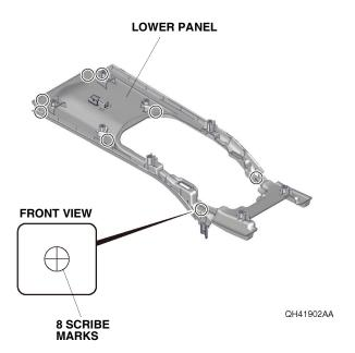
If the vehicle is equipped with eight scribe marks, go to step 28; otherwise, continue with step 24.
