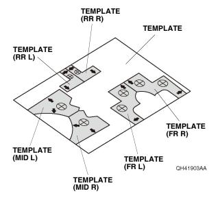
25. Place the four templates on the lower panel as shown. Secure the four templates to the lower panel with masking tape.
