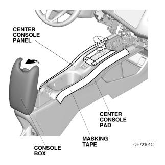
Apply masking tape to the center console panel and center console pad as shown.
