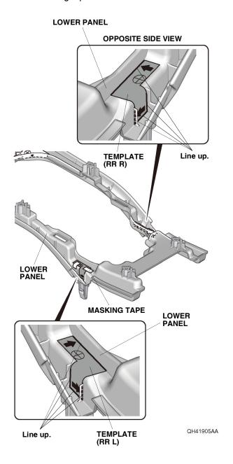
27. Using a pushpin, pierce the lower panel as shown. Remove the six templates. Go to step 29. NOTE: Make sure to pierce the printed marks perpendicular to the lower panel.
