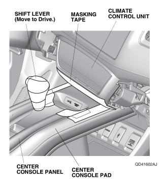
10. Remove the center console switch trim, and unplug the vehicle connector.
