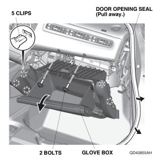
6. Pull away the door opening seal, and remove the driver's dashboard side lid.
