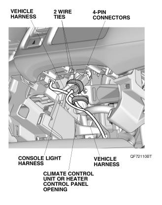
39. Secure the 2-pin connectors to the center console pad with one wire tie with clip as shown. If the vehicle already has a harness there, cut the clip portion off the wire tie and secure the 2-pin connector to the other harness as shown.
