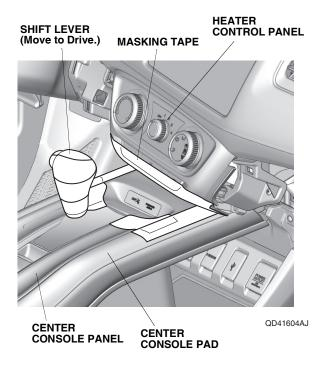
14. Remove the center console switch trim, and unplug the vehicle connector.
