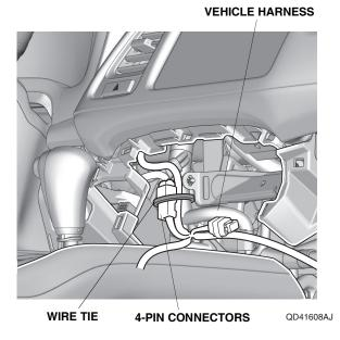
22. Route the ambient light harness as shown. Line up the green tape on the ambient light harness with the vehicle clip, and secure the ambient light harness to the vehicle harness with three wire ties.
