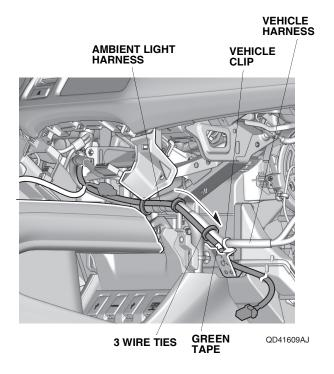
23. Route the ambient light harness as shown. Secure the ambient light harness to the vehicle harness with two wire ties.
