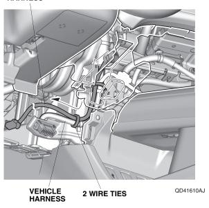
24. Secure the ambient light harness to the vehicle harness with two wire ties.
