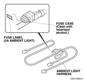
19. Attach the fuse label (2A AMBIENT LIGHT) to the fuse case on the ambient light harness.
