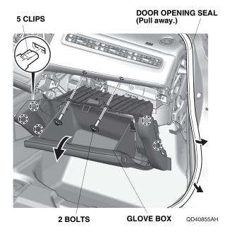
7. Pull away the door opening seal, and remove the driver's dashboard side lid.
