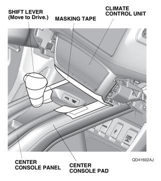
11. Remove the center console switch trim, and unplug the vehicle connector.
