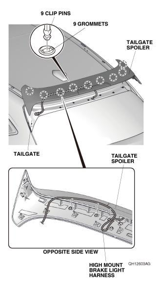
4. Disconnect the rear washer tube. Remove the grommet on the high mount brake light harness from the vehicle panel, and unplug the vehicle connector. Place the tailgate spoiler on a blanket.
