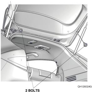
3. With the help of an assistant, carefully pull on the tailgate spoiler to release the nine clip pins from the grommets. Release the high mount brake light harness.
