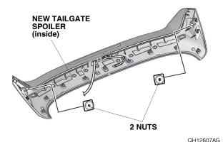
13. Secure the high mount brake light harness to the new tailgate spoiler.
