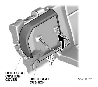
16. Secure the right seat cushion cover to the right seat cushion with the two hooks and two loops, and lower the right seat cushion.
