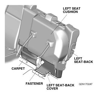
5. Lower the left seat cushion and fold the left seat-back fully forward. Pull the seat-back cover tight and secure it to the left seat-back with five fasteners.
