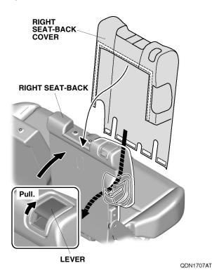
11. Lift up the right seat cushion. Secure the fastener on the right seat-back cover as shown.
