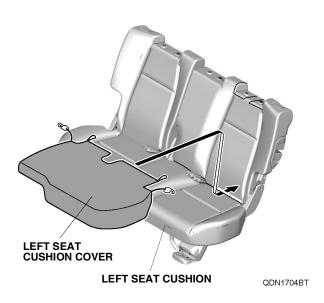
8. Lift up the left seat cushion. Secure the fasteners on the left seat cushion cover as shown.
