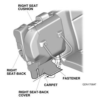
12. Lower the right seat cushion, and fold the right seat-back fully forward. Pull the seat-back cover tight, and secure it to the right seat-back with four fasteners.
