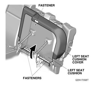
Secure the left seat cushion cover to the left seat cushion with the two hooks and two loops, and lower the left seat cushion.
