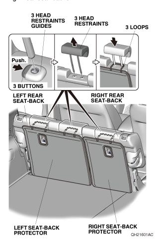
2. Fold down the left and right rear seat-backs, and peel back the cargo floor lid. Line up the left and right seat-back protectors with the tether anchor covers on the left and right rear seat-backs as shown. Secure the left and right seat-back protectors to the left and right rear seat-backs with the 28 fasteners.
