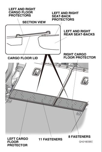
4. Check the protectors by moving the left and right rear seat-backs back and forth.
