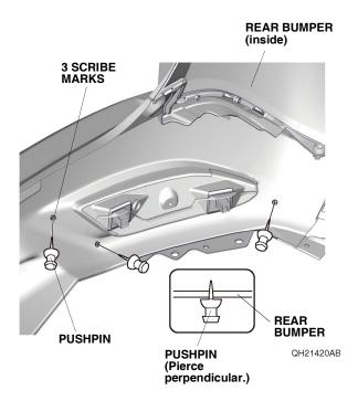
3. While wearing eye protection, drill this pierced marks to 4 mm. Remove all burrs. Repeat on the right side of the rear bumper.
