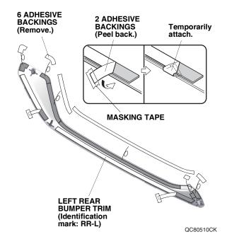
Loosely install the left rear bumper trim to the rear bumper with two spacers, two washers, and two selftapping screws.
