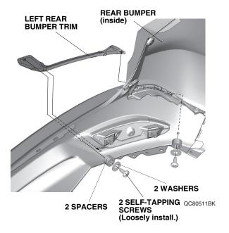
8. While applying light pressure against the left rear bumper trim, carefully remove the adhesive backings.
