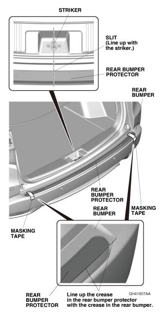
2. On the right side of the rear bumper protector, line up the crease in the bumper protector with the crease in the bumper. Then, secure the rear bumper protector to the rear bumper with masking tape, and repeat this on the left side.
