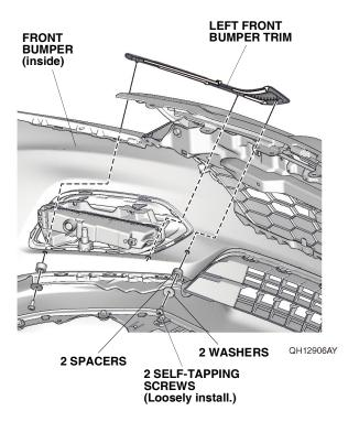
9. While applying light pressure against the left front bumper trim, carefully remove the adhesive backings.
