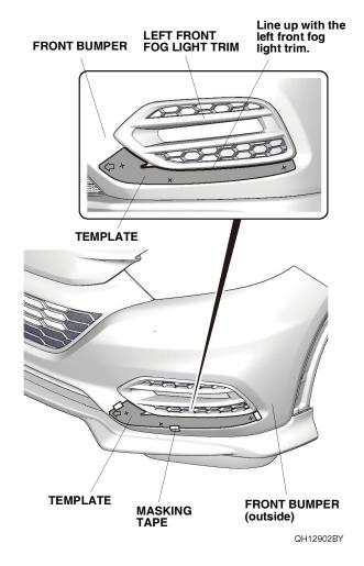
4. Using a pushpin, pierce the three marks in the template on the front bumper.
