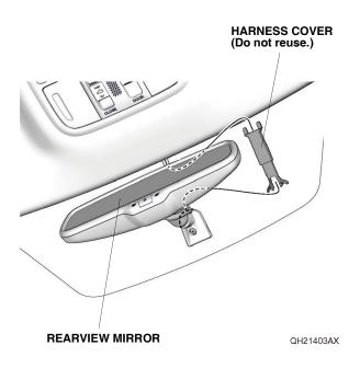
3. Loosen the TORX screw. Remove the rearview mirror, and unplug the vehicle connector. Go to step 5.
