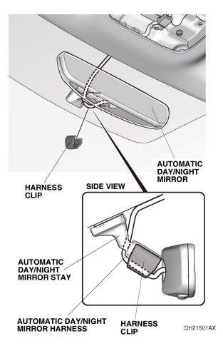
33. Route the automatic day/night mirror harness through the groove in the harness cover. Secure the harness cover to the automatic day/night mirror stay. Slide the harness cover behind the headliner. Go to step 35.
