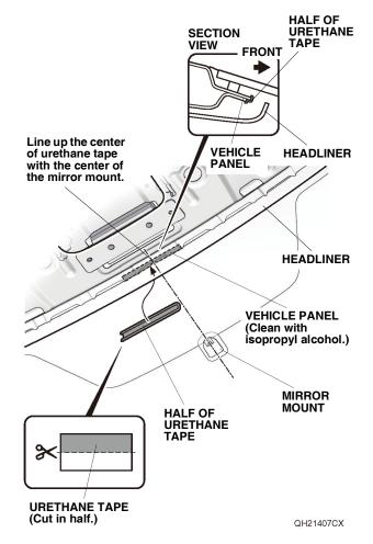
Using scissors, cut one piece of urethane tape in half. Attach the one piece to the vehicle panel as shown.
