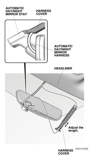
35. Route the automatic day/night mirror harness down the A-pillar as shown. Line up the green tape on the automatic day/night mirror harness with the vehicle clip, and secure the automatic day/night mirror harness to the vehicle harness with one wire tie. NOTE: Do not cover the installation holes of the driver's A-pillar trim.
