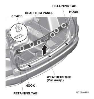
10. Pull away the weatherstrip and the door opening seal. Remove the left rear side trim panel and unplug the vehicle connector, if equipped.
