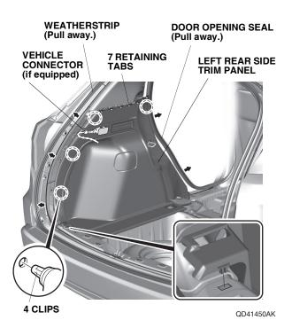
11. Pull away the weatherstrip and the door opening seal. Remove the right rear side trim panel.
