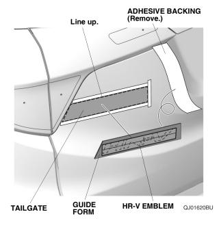
23. Remove the guide form and using the palm of your hand, firmly press the HR-V emblem against the tailgate.
