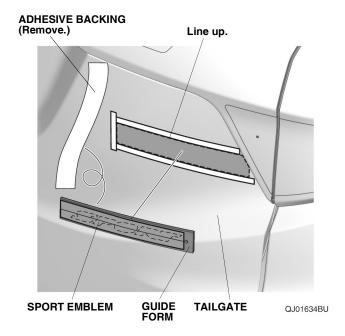
40. Remove the guide form and using the palm of your hand, firmly press the SPORT emblem against the tailgate.
