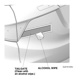
22. Remove the adhesive backing from the HR-V emblem. Line up the guide form with the masking tape, and attach the HR-V emblem to the tailgate.
