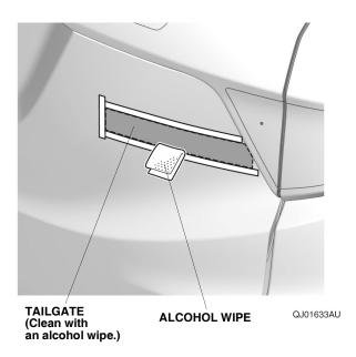
39. Remove the adhesive backing from the SPORT emblem. Line up the guide form with the masking tape, and attach the SPORT emblem to the tailgate.
