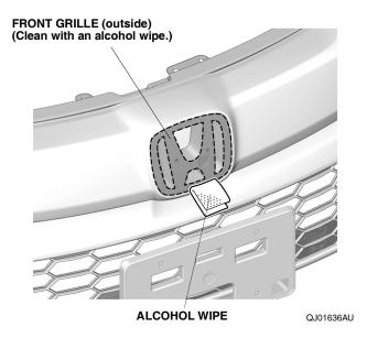
7. Remove the adhesive backings from the front H emblem. Install the front H emblem to the front grille as shown.
