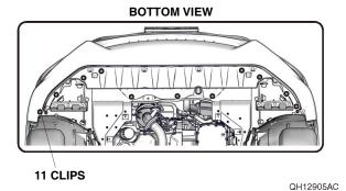
Remove the two self-tapping screws and four clips on each side.
