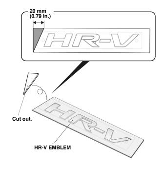
5. Remove the position film from the HR-V emblem, then remove the HR-V emblem from the guide form.
