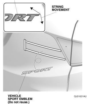
37. Install the SPORT emblem in the guide form, and temporarily secure it with masking tape.
