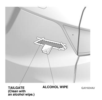
28. Remove the adhesive backing from the AWD emblem. Line up the AWD emblem with the masking tape, and attach the AWD emblem to the tailgate.
