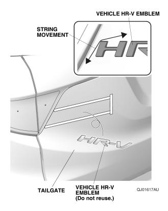
20. Install the HR-V emblem in the guide form, and temporarily secure it with masking tape.
