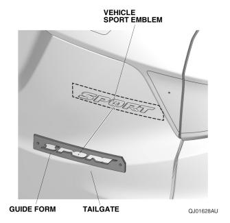
34. Attach masking tape along the guide form as shown.
