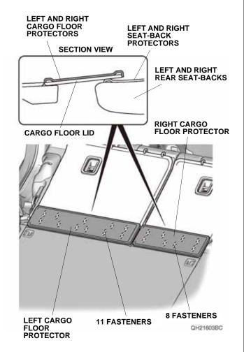
4. Check the protectors by moving the left and right rear seat-backs back and forth.
