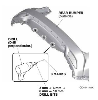
4. While wearing eye protection, drill the 10 pierced marks to 6 mm. First, drill with a 3 mm drill bit, and finish with a 6 mm drill bit. Remove all burrs. NOTE: Make sure to drill perpendicular to the rear bumper.
