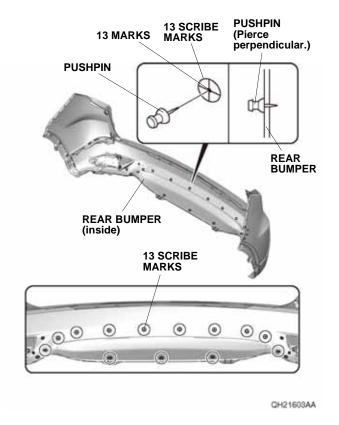
3. While wearing eye protection, drill these three pierced marks to 10 mm. First, drill with a 3 mm drill bit, then follow with a 6 mm drill bit and 8 mm drill bit, and finish with a 10 mm drill bit. Remove any burrs. NOTE: Make sure to drill perpendicular to the rear bumper.
