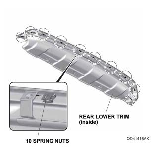
6. Install the rear lower trim to the rear bumper with three clips.
