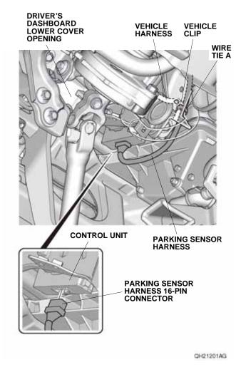
69. Secure the parking sensor harness to the vehicle harness with one wire tie A.
