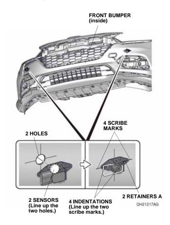
98. Make sure the two sensors are installed properly.
