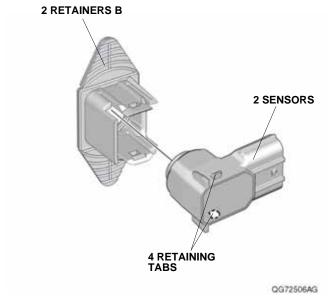
121. Line up the two sensors and two retainers B to the rear bumper as shown.
