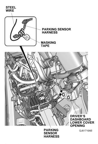
60. Route the parking sensor harness as shown. Remove the masking tape and steel wire.
