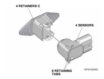
150. Line up the four sensors and four retainers C to the rear bumper as shown.
