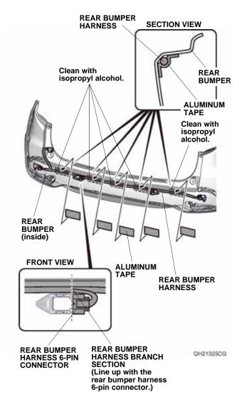
136. Line up the branch section of the rear bumper harness with the rear bumper harness 6-pin connector. Secure the rear bumper harness to the rear bumper with five pieces of aluminum tape as shown. Go to step 140.
