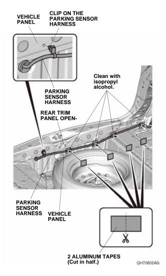
80. Using scissors, cut two aluminum tapes in half, and secure the parking sensor harness to the vehicle panel with the clip on the parking sensor harness and four pieces of aluminum tape as shown.
