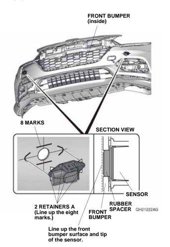
102. Remove the two sensors, and firmly press the two retainers A against the front bumper.
