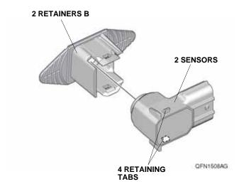
119. Using diagonal cutters, cut the tabs off the two retainers B as shown. Remove any burrs.
