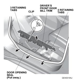
22. Pull away the door opening seal, and remove the driver's kick panel.
