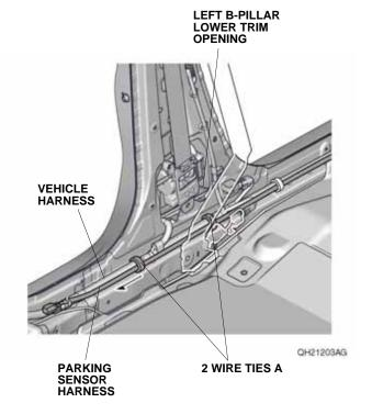
72. Route the parking sensor harness along the vehicle harness, and secure it to the vehicle harness with three wire ties A as shown.
