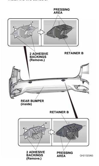
133. Make sure the four sensors are installed properly.
