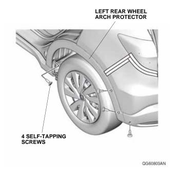
Remove the rear wheel arch protector on each side.
