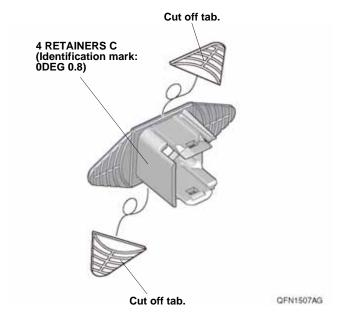
149. Install the four sensors to the four retainers C.
