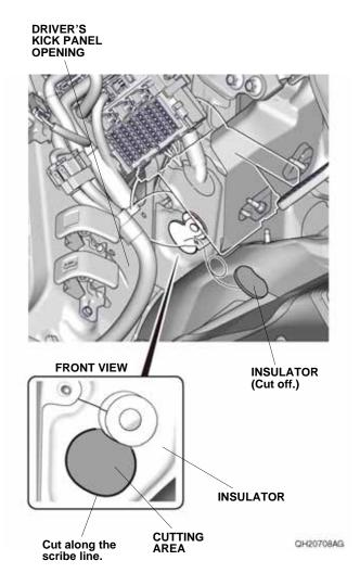
36. Remove the vehicle grommet. Route the subharness through the vehicle panel hole as shown.
