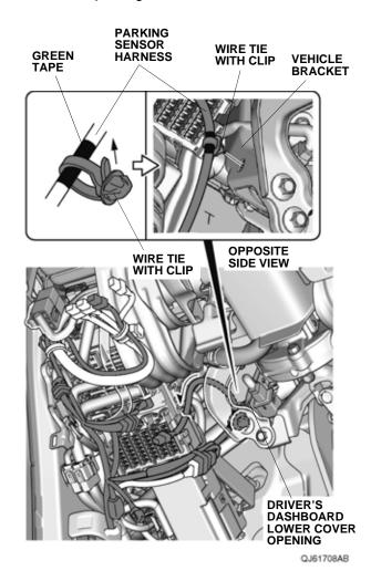
49. Attach one wire tie with clip around the green tape on the parking sensor harness as shown. Secure the parking sensor harness to the vehicle bracket with one wire tie with clip. Go to step 53.
