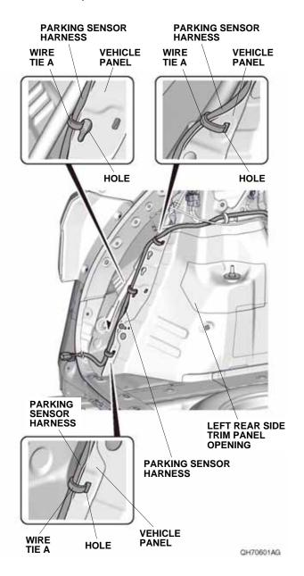
76. Remove the vehicle grommet. Route the parking sensor harness through the vehicle panel hole as shown
