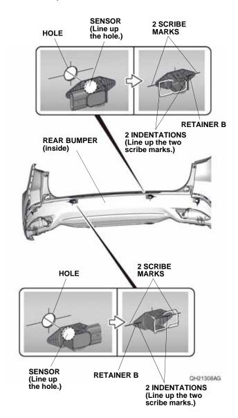
123. Make sure the four sensors are installed properly.
