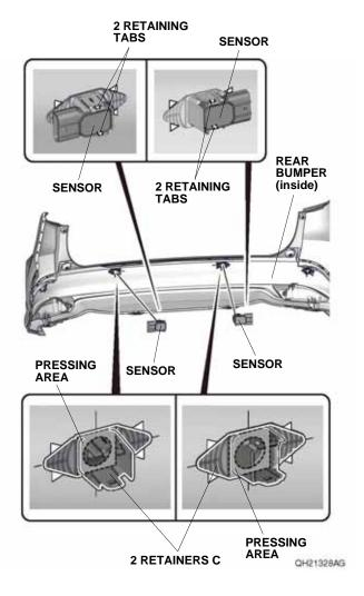
157. Remove the eight adhesive backings, and firmly press the four retainers C against the rear bumper. Install the four sensors.
