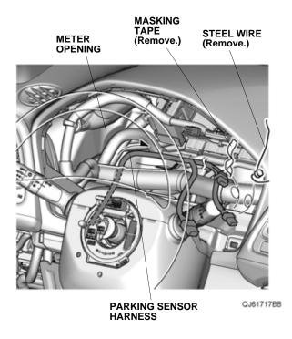
61. Secure the parking sensor harness to the vehicle harness with three wire ties A.
