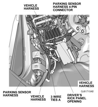
54. Plug the subharness 4-pin connector into the parking sensor harness 4-pin connector.
