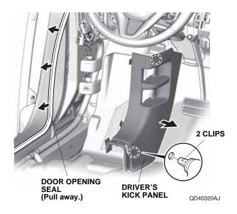
23. Pull away the door opening seal, and remove the left rear door sill trim.
