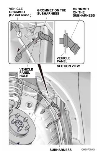
37. Secure the grommet on the subharness to the vehicle panel hole.
