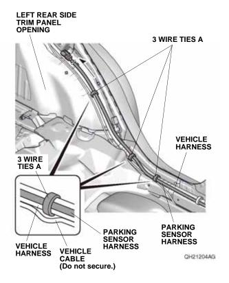
73. Route the parking sensor harness along the vehicle harness, and secure it to the vehicle harness with three wire ties A.
