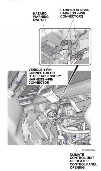
65. Secure the parking sensor harness to the vehicle harness with one wire tie A.
