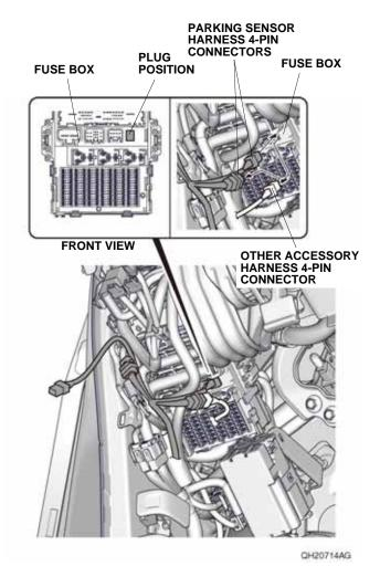
43. Plug the other accessory harness 4-pin connector into the parking sensor harness 4-pin connector.
