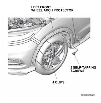
Remove the front wheel arch protector on each side.
