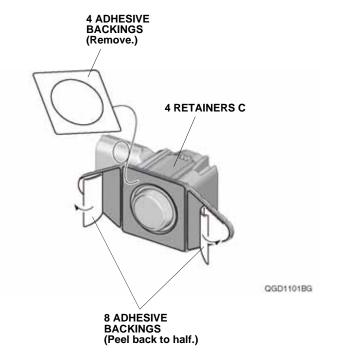
154. Attach the four retainers C to the rear bumper as shown.
