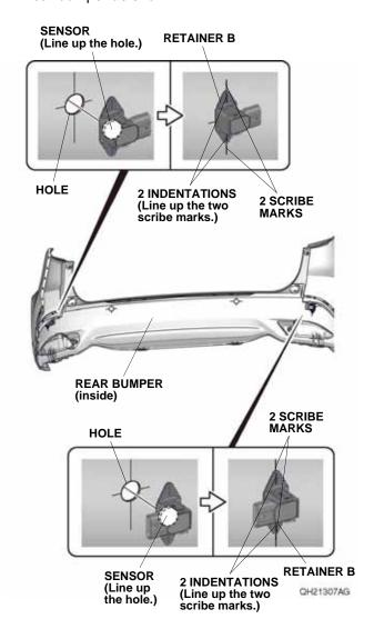
122. Line up the two sensors and two retainers B to the rear bumper as shown.
