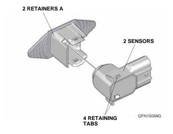
97. Line up the two sensors and two retainers A to the front bumper as shown.
