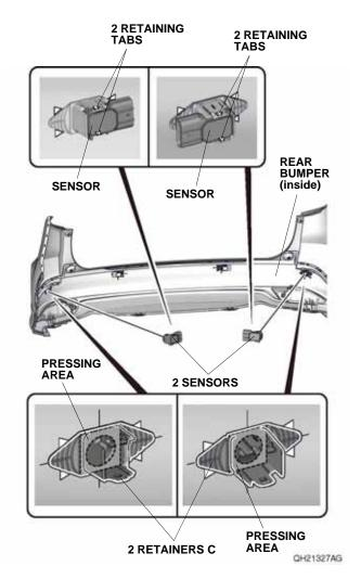
156. Remove the two sensors, and firmly press the two retainers C against the rear bumper.
