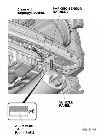
85. Using scissors, cut one aluminum tape in half, and secure the parking sensor harness to the vehicle panel with one piece of aluminum tape as shown.
