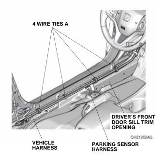
71. Route the parking sensor harness along the vehicle harness, and secure it to the vehicle harness with two wire ties A as shown.
