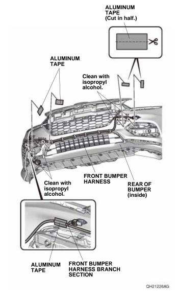
108. Secure one side of the front bumper harness to the bumper with two pieces of aluminum tape. Using scissors, cut one piece of aluminum tape in half, and secure the front bumper harness to the other side of the front bumper with those two pieces of aluminum tape as shown.
