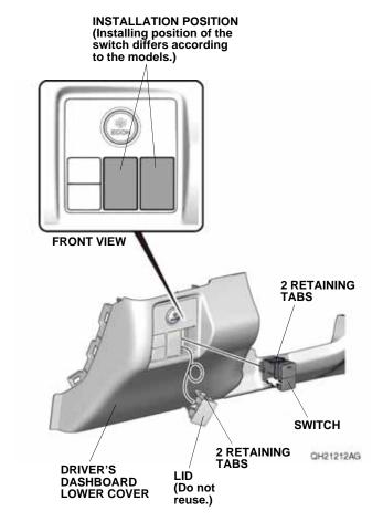
87. Install the switch to the driver's dashboard lower cover.
