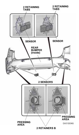
130. Remove the two sensors, and firmly press the two retainers B against the rear bumper.
