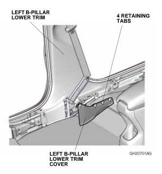
25. Pull away the door opening seal, and remove the left B-pillar lower trim.
