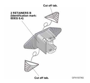
118. Install the two sensors to the two retainers B.
