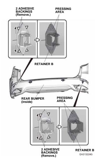
132. Remove the four adhesive backings, and firmly press the two retainers B against the rear bumper. Install the two sensors.
