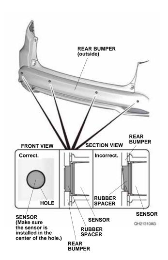
152. Using a felt-tip pen, mark the rear bumper as shown.
