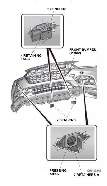
103. Remove the four adhesive backings, and firmly press the two retainers A against the front bumper. Install the two sensors.
