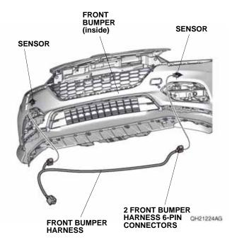
106. Secure the front bumper harness to the front bumper lower grille with six wire ties B (narrow) as shown.
