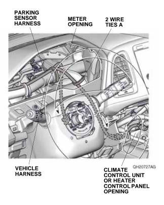
63. Secure the parking sensor harness to the vehicle harness with two wire ties A.
