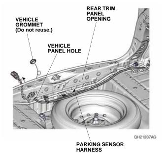
77. Secure the grommet on the parking sensor harness to the vehicle panel hole.
