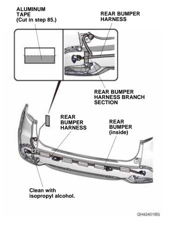
141. Secure the rear bumper harness to the rear bumper with one piece of aluminum tape cut in step 85 as shown. Go to step 167.
