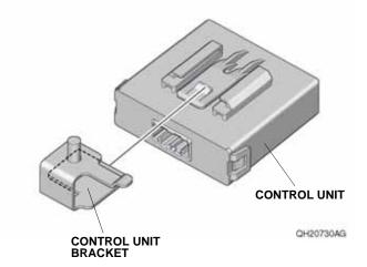
67. Install the control unit to the vehicle frame with one washer nut.
