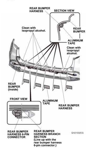
161. Line up the branch section of the rear bumper harness with the rear bumper harness 6-pin connector. Secure the rear bumper harness to the rear bumper with five pieces of aluminum tape as shown. Go to step 165.
