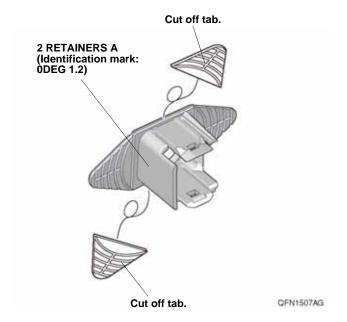
96. Install the two sensors to the two retainers A.
