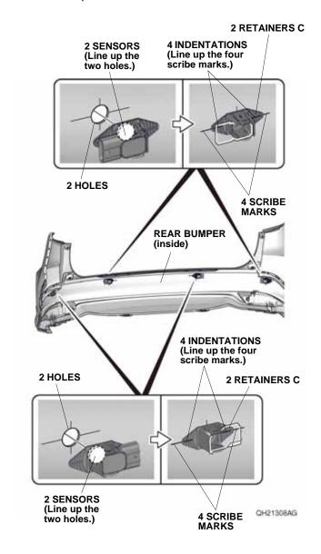
151. Make sure the four sensors are installed properly.
