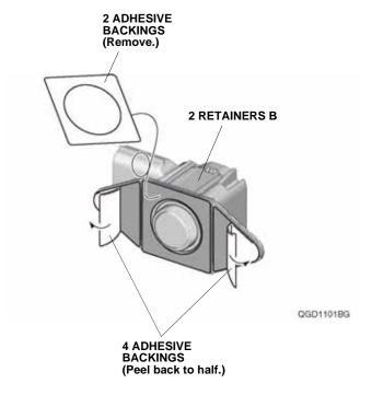
128. Attach the two retainers B to the rear bumper as shown.
