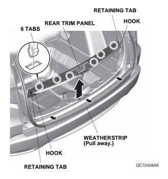
31. Pull away the weatherstrip and door opening seal. Remove the left rear side trim panel, and unplug the vehicle connector (if equipped).
