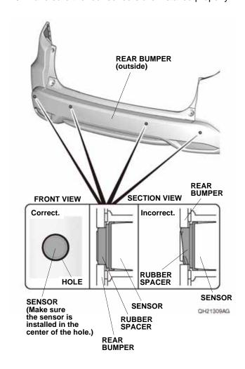
124. Using a felt-tip pen, mark the rear bumper as shown.
