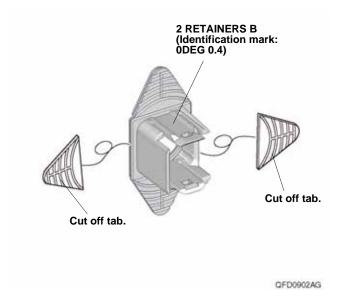
120. Install the two sensors to the two retainers B.
