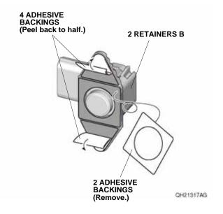
126. Attach the two retainers B to the rear bumper as shown.
