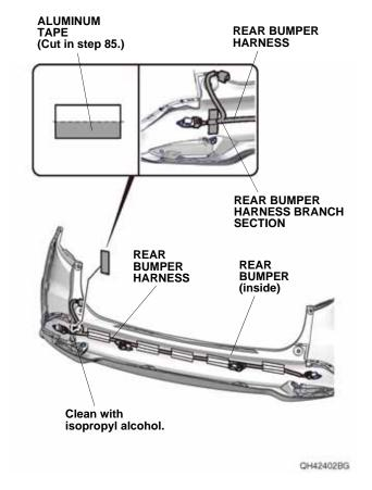
166. Secure the rear bumper harness to the rear bumper with one piece of aluminum tape cut in step 85 as shown.
