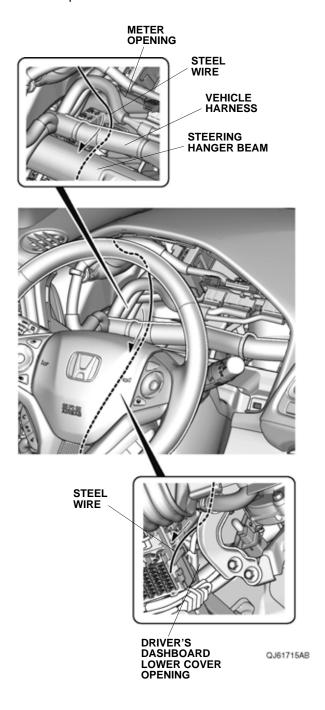
59. Attach the steel wire to the parking sensor harness with masking tape as shown.
