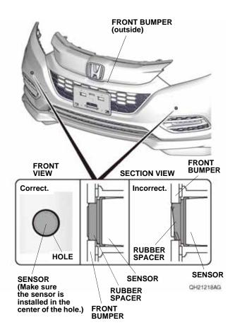
105. Plug the two front bumper harness 6-pin connectors into the two sensors.
