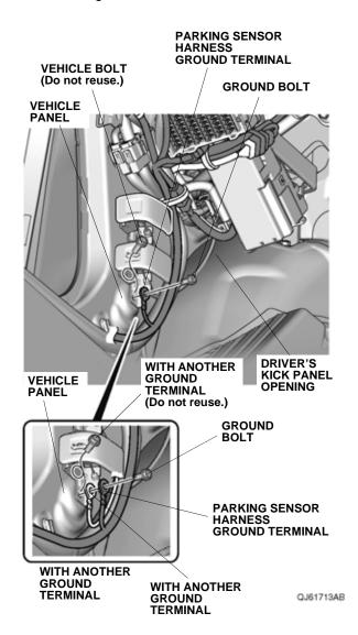
57. Secure the parking sensor harness to the vehicle harness with two wire ties A.
