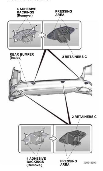
158. Make sure the four sensors are installed properly.
