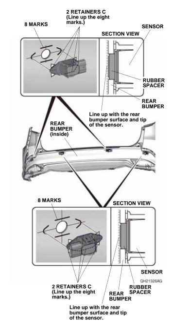
155. Remove the two sensors, and firmly press the two retainers C against the rear bumper.
