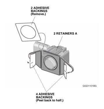
101. Attach the two retainers A to the front bumper as shown.
