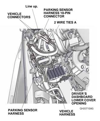
45. Secure the parking sensor harness to the vehicle harness with two wire ties A.
