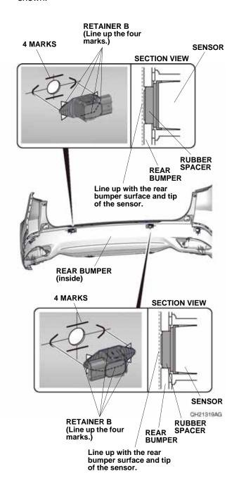
129. Remove the two sensors, and firmly press the two retainers B against the rear bumper.
