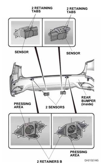
131. Remove the four adhesive backings, and firmly press the two retainers B against the rear bumper. Install the two sensors.
