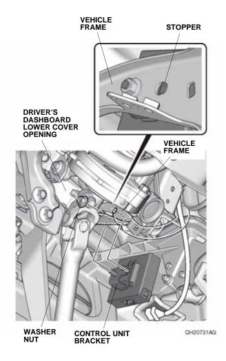
68. Plug the parking sensor harness 16-pin connector into the control unit.
