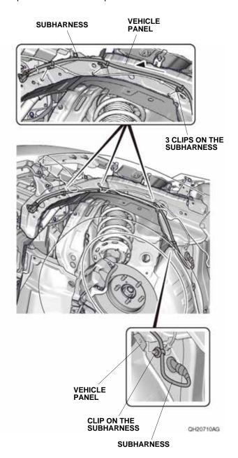
39. Secure the subharness 4-pin connector to the vehicle panel with the clip on the subharness 4-pin connector.
