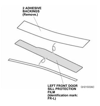
5. Spray the left front door sill protection film with the 3M protective tape application solution.
