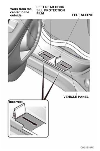
21. Gently bend the left rear door sill protection film around the radius on the vehicle panel using your hand. Repeat until the film is attached to the vehicle panel. Repeat step 19 to set the adhesive of the left rear door sill protection film to the radius and the edge of the vehicle panel.
