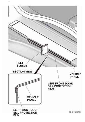
12. Using a shop towel, wipe off the 3M protective tape application solution. Allow the left front door sill protection film to dry thoroughly. Remove the masking tape.
