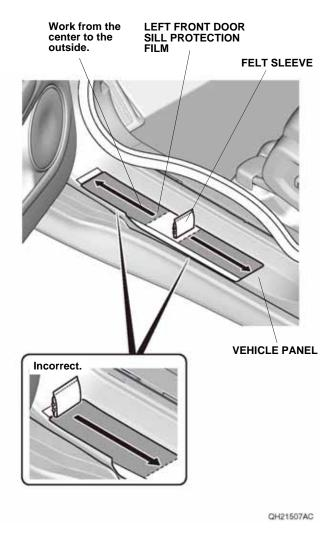
10. Gently bend the left front door sill protection film around the radius on the vehicle panel using your hand. Repeat until the film is attached to the vehicle panel. Repeat step 8 to set the adhesive of the left front door sill protection film to the radius and the edge of the vehicle panel.
