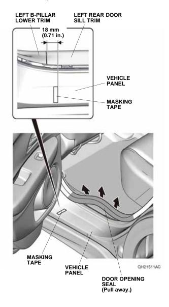
Using an alcohol wipe, thoroughly clean the vehicle panel where the left rear door sill protection film will attach.
