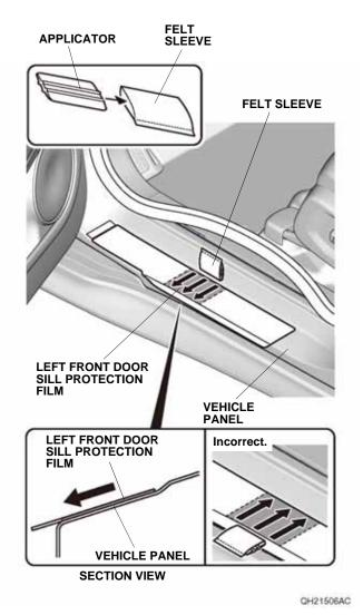
8. Starting from the inside and working outside, use the felt sleeve to smooth out the center of the left front door sill protection film. Move the felt sleeve in one direction only. If you see an air bubble, stop and gently peel up that section to work out the bubble. Work slowly, and keep pressure against the left front door sill protection film.
