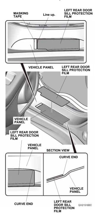
19. Starting from the inside and working outside, use the felt sleeve to smooth out the center of the left rear door sill protection film. Move the felt sleeve in one direction only. If you see an air bubble, stop and gently peel up that section to work out the bubble. Work slowly, and keep pressure against the left rear door sill protection film.
