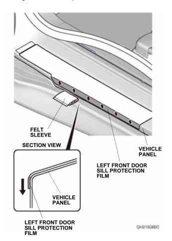
11. Repeat step 9 to set the adhesive of the left front door sill protection film to the edge of the vehicle panel.
