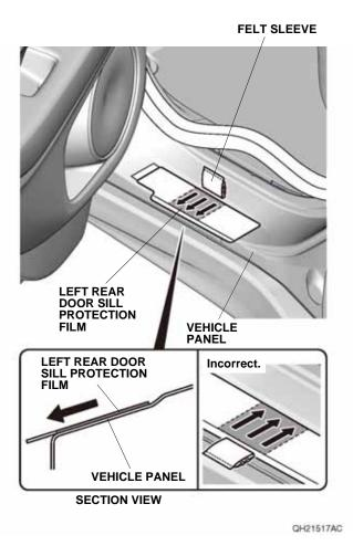
20. Starting from the center and working outward, use the felt sleeve to smooth out the left and right sides of the upper section on the left rear door sill protection film. Move the felt sleeve in one direction only. If you see an air bubble, stop and gently peel up that section to work out the bubble. Work slowly, and keep pressure against the left rear door sill protection film.
