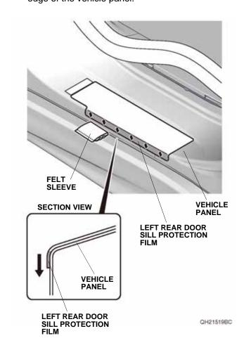
22. Repeat step 20 set the adhesive of the left rear door sill protection film to the edge of the vehicle panel.
