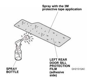
18. Line up the left rear door sill protection film with the curve end and masking tape as shown. Attach the left rear door sill protection film to the vehicle panel. NOTE: Be careful not to overlap on the curve end.
