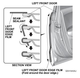
8. Using a shop towel, to wipe the excess 3M protective tape application solution from the left front door edge film. Allow the left front door edge film to dry thoroughly.
