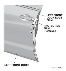
7. Starting from the center and working outward, use your fingers to fold the left front door edge film around the edge of the left front door as shown. Move your fingers in one direction only. Attach the left front door edge film over the seam sealant. Do not trim or damage the seam sealant.
