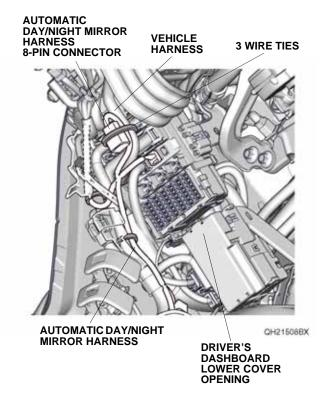
45. Route the automatic day/night mirror harness along the vehicle harness. Remove the bolt, and secure the automatic day/night mirror harness ground terminal to the vehicle panel with one ground bolt. If the vehicle is equipped with another accessory harness ground terminal, remove the other accessory harness ground bolt, and secure the other accessory harness ground terminal and automatic day/night mirror harness ground terminal to the vehicle panel with one ground bolt.
