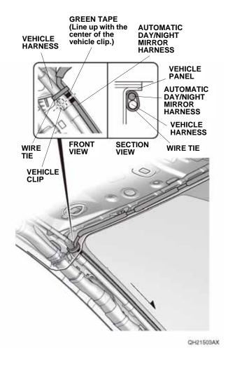
36. Line up the green tape on the automatic day/night mirror harness with the vehicle clip, and secure the automatic day/night mirror harness to the vehicle harness with one wire tie.
