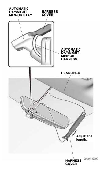
35. Route the automatic day/night mirror harness down the A-pillar as shown. Line up the green tape on the automatic day/night mirror harness with the vehicle clip, and secure the automatic day/night mirror harness to the vehicle harness with one wire tie. NOTE: Do not cover the installation holes of the driver's A-pillar trim.
