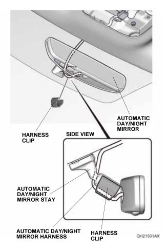
33. Route the automatic day/night mirror harness through the groove in the harness cover. Secure the harness cover to the automatic day/night mirror stay. Slide the harness cover behind the headliner. Go to step 35.
