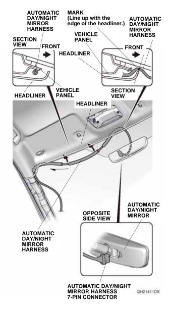
31. Gently pull back the headliner, and tuck the automatic day/night mirror harness behind the headliner. Line up the mark on the automatic day/night mirror harness with the edge of the headliner. NOTE: Be careful not to crease the headliner.
