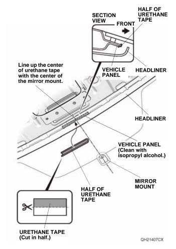
20. Using scissors, cut one piece of urethane tape in half. Attach the one piece to the vehicle panel as shown.
