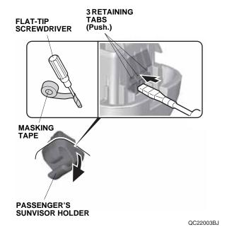
While holding down the passenger's sunvisor holder as shown, use a flat-tip screwdriver wrapped with masking tape to remove the passenger's sunvisor holder.
