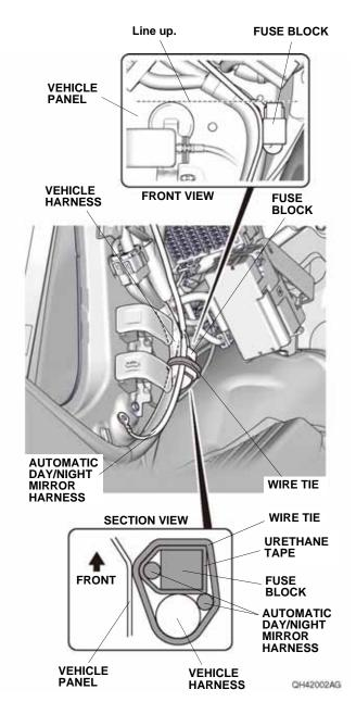
44. Secure the automatic day/night mirror harness 8-pin connector and automatic day/night mirror harness to the vehicle harness with three wire ties.
