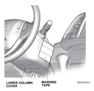
8. Pull away the door opening seal. Remove the driver's dashboard lower cover, and unplug the vehicle connectors.
