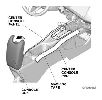
18. Apply masking tape to the center console panel and center console pad as shown.
