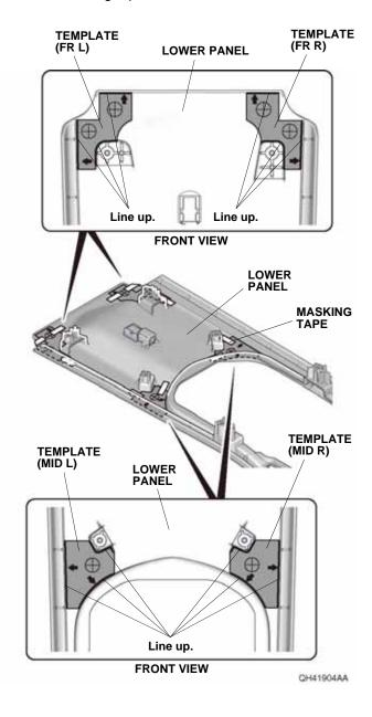
26. Place the two templates on the lower panel as shown. Secure the two templates to the lower panel with masking tape.
