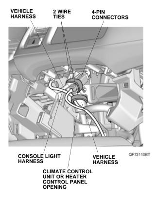
39. Secure the 2-pin connectors to the center console pad with one wire tie with clip as shown. If the vehicle already has a harness there, cut the clip portion off the wire tie and secure the 2-pin connector to the other harness as shown.
