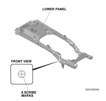
If the vehicle is equipped with eight scribe marks, go to step 28; otherwise, continue with step 24.
