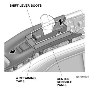
21. Remove the center console pad, and unplug the vehicle connector (if equipped).
