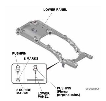
29. While wearing eye protection, drill the eight pierced marks on the lower panel to 6 mm. First, drill with a 3 mm drill bit, then finish with a 6 mm drill bit. NOTE: Make sure to drill perpendicular to the lower panel.
