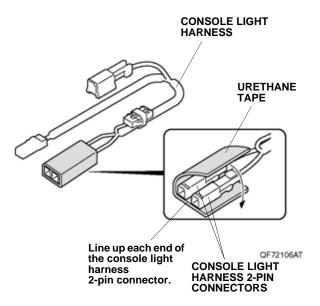
35. Plug the left light 2-pin connector and right light 2-pin connector into the console light harness 2-pin connectors.
