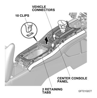
20. Release the shift lever boots, and remove the center console panel.
