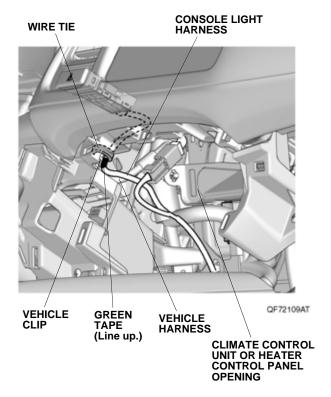
38. Secure the console light harness and 4-pin connectors to the vehicle harness with two wire ties.
