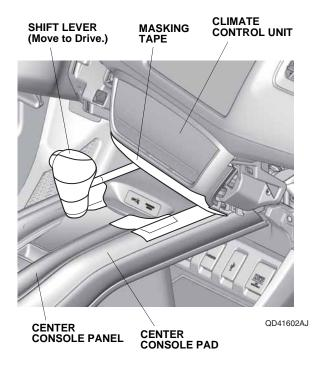
10. Remove the center console switch trim, and unplug the vehicle connector.
