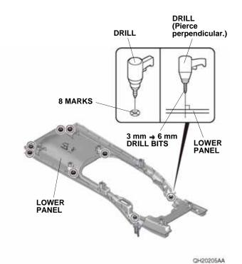
30. While wearing eye protection, drill the six holes on the lower panel to 10 mm as shown. First, drill with an 8 mm drill bit, then finish with an 10 mm drill bit. Remove any burrs.
