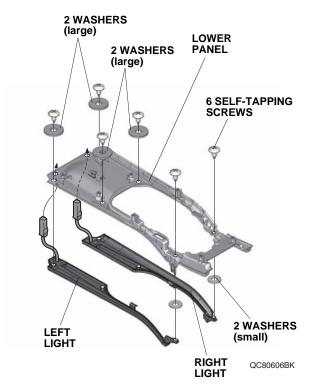
32. Install the lower panel, pad bracket, and center console pad.
