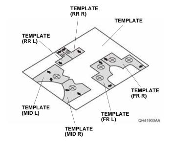
25. Place the four templates on the lower panel as shown. Secure the four templates to the lower panel with masking tape.
