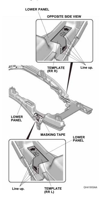
27. Using a pushpin, pierce the lower panel as shown. Remove the six templates. Go to step 29. NOTE: Make sure to pierce the printed marks perpendicular to the lower panel.
