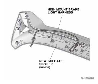
14. Plug the vehicle 2-pin connector into the high mount brake light harness 2-pin connector, and install the grommet on the high mount brake light harness to the vehicle panel hole.
