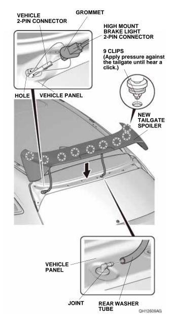
15. Connect the rear washer tube to the joint. Install the new tailgate spoiler to the tailgate with nine clips. NOTE: To confirm clip engagement, listen for a click sound during installation.
