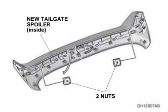
13. Secure the high mount brake light harness to the new tailgate spoiler.
