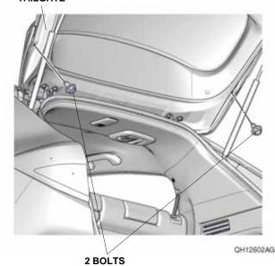
With the help of an assistant, carefully pull on the tailgate spoiler to release the nine clip pins from the grommets. Release the high mount brake light harness.
