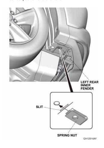
6. Secure the left rear splash guard with two 5 x 25 mm self-tapping screws and one 5 x 18 mm self-tapping screw in the order shown below.
