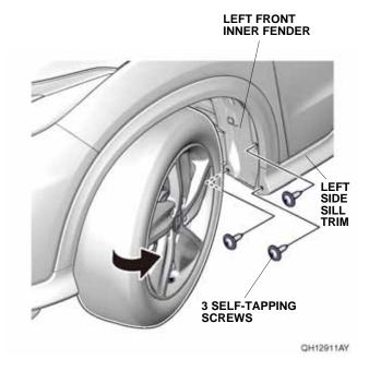
2. Remove the three self-tapping screws.
