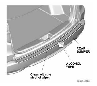
Peel back the adhesive backings, and tape them to the front surface of the rear bumper protector with masking tape. Remove the remaining adhesive backings.
