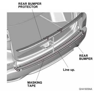
8. While applying light pressure to the rear bumper protector, carefully remove the taped adhesive backings as shown.
