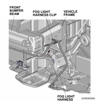
25. Secure the fog light harness to the vehicle harness with one wire tie.
