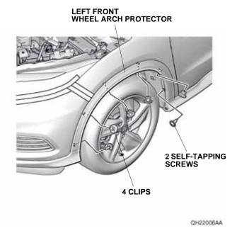
Remove the front wheel arch protector on each side.
