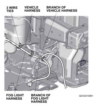
23. Secure the fog light harness clip to the hole in the vehicle frame as shown.
