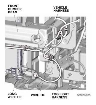
31. Connect two long wire ties together, and secure the fog light harness to the front bumper beam with them.
