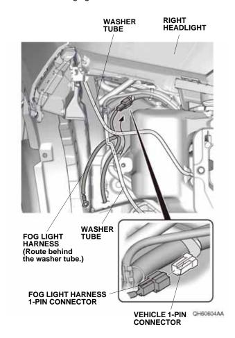
18. Plug the vehicle 1-pin connector into the fog light harness 1-pin connector.
