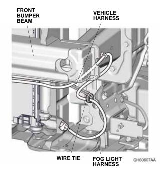
26. Connect two long wire ties together, and secure the fog light harness to the front bumper beam with them. Go to step 32.
