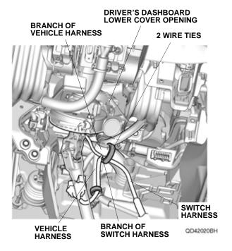
Secure the switch harness to the vehicle harness with three wire ties.
