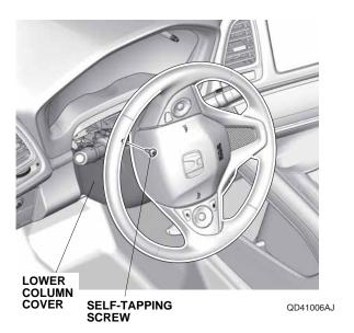
7. Turn the steering wheel 180° clockwise, and remove the self-tapping screw from the lower column cover.
