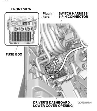
46. Secure the switch harness to the vehicle harness with one wire tie.
