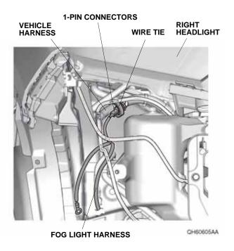
20. Route the fog light harness as shown. Install the fog light harness ground terminal to the vehicle panel with one ground bolt.
