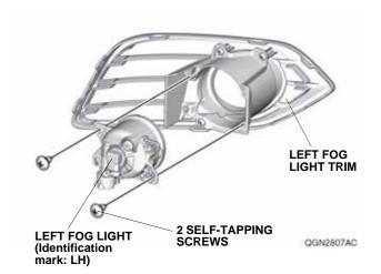
15. Install the left fog light trim to the front bumper with nine retaining tabs.
