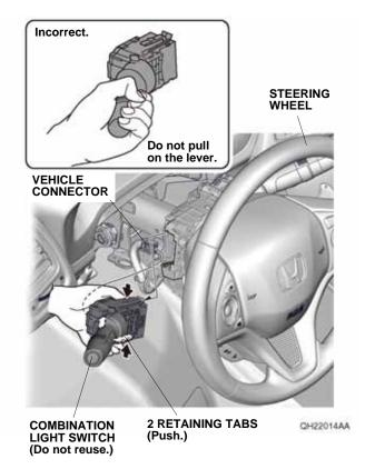
48. While pushing the two retaining tabs, slide the combination light switch out and remove it from the steering column.
