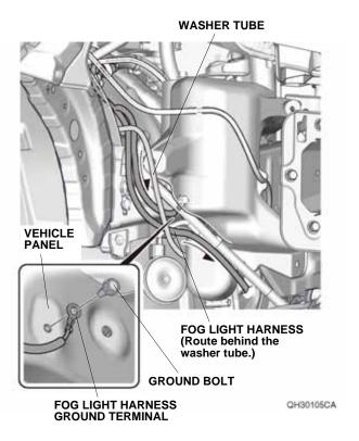
21. Secure the fog light harness to the vehicle harness with one wire tie.
