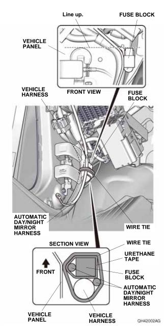
44. Secure the automatic day/night mirror harness 8-pin connector and automatic day/night mirror harness to the vehicle harness with three wire ties.
