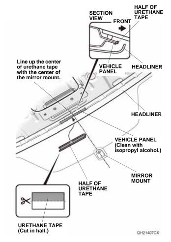
Using scissors, cut one urethane tape in half. Attach
