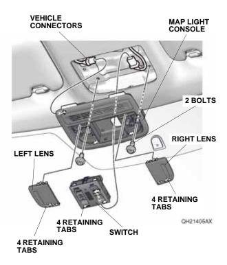
Without moonroof: Remove the map light console, and unplug the vehicle connectors.
