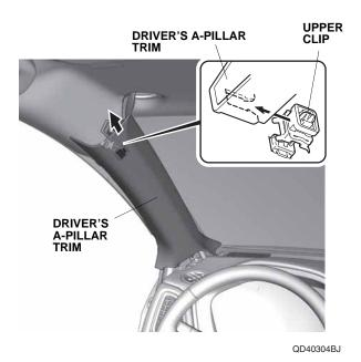
12. Remove the remaining upper clip from the driver's A-pillar.
