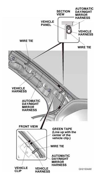
37. Secure the automatic day/night mirror harness to the vehicle harness with one wire tie.
