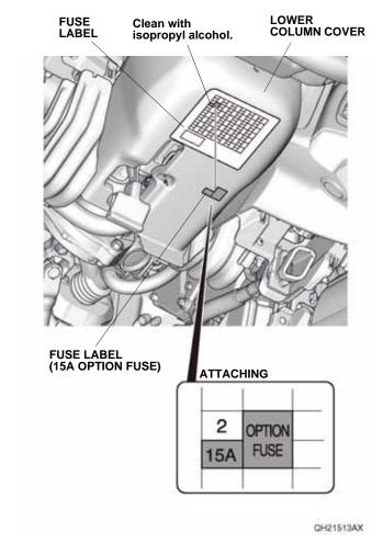
49. Attach the fuse label (15A OPTION FUSE) to the fuse label on the lower column cover as shown.
