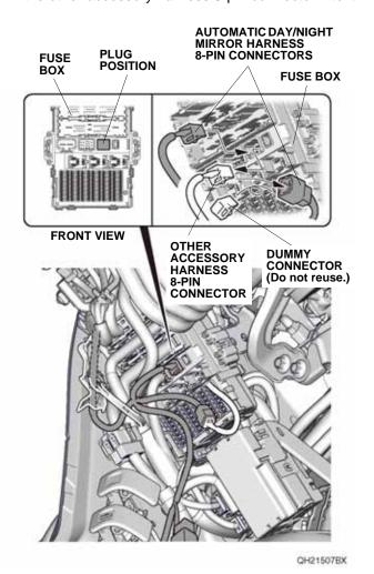
43. Secure the fuse block on the automatic day/night mirror harness and automatic day/night mirror harness to the vehicle harness with one wire tie.
