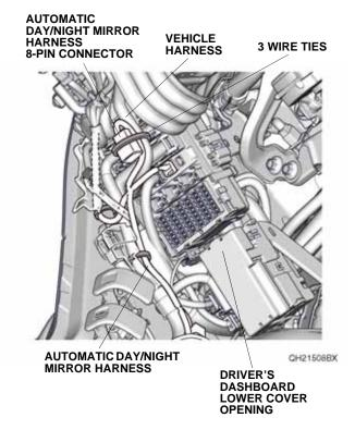
45. Route the automatic day/night mirror harness along the vehicle harness. Remove the bolt, and secure the automatic day/night mirror harness ground terminal to the vehicle panel with one ground bolt. If the vehicle is equipped with another accessory harness ground terminal, remove the other accessory harness ground bolt, and secure the other accessory harness ground terminal and automatic day/night mirror harness ground terminal to the vehicle panel with one ground bolt.
