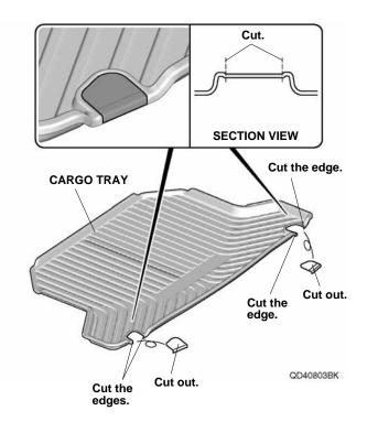
5. Open the tailgate. Place the cargo tray on the cargo floor.
