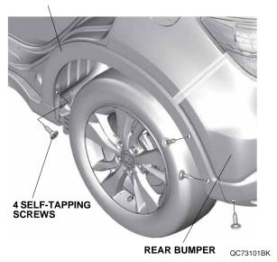
Remove the rear wheel arch protector on each side.
