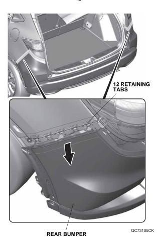
With the help of an assistant, remove the rear bumper. Place the rear bumper on the blanket to prevent damage.
