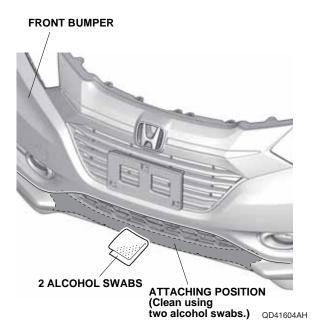
7. Peel back about 40 to 50 mm (1.5 to 2.0 in.) of adhesive backing from each adhesive strip, and tape the ends to the front surface of the front lower trim. Remove the other adhesive backings.
