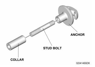
20. Install the EPT sealer onto anchor and thread the rivet nut onto the stud bolt. Adjust the anchor as shown.
