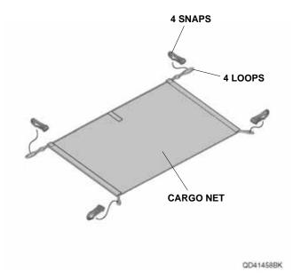
Attach the four snaps on the cargo net to the tie-down hooks as shown.
