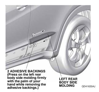
11. Using the rubber roller, apply firm pressure while rolling to set the adhesive. Apply firm pressure especially at the ends.
