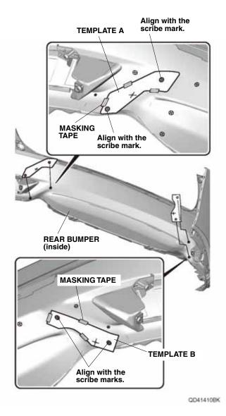
3. Using a pushpin, pierce the rear bumper at the mark on template A as shown.
