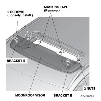
12. Position the moonroof visor with equal spacing in the front and on the sides. Check that the rubber molding is not twisted or rolled under the moonroof visor.
