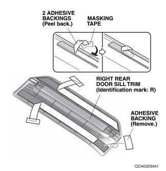
58. Using an alcohol swab, clean the vehicle panel where the right rear door sill trim will attach.
