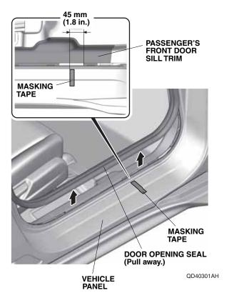
3. Remove the passenger's front door sill trim.
