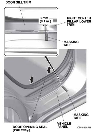
57. Peel back the ends of two adhesive backings on the right rear door sill trim and attach them to the front of the trim with masking tape. Remove one adhesive backing.
