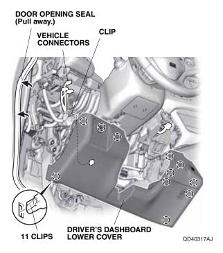
13. Pull away the door opening seal, and attach masking tape to the vehicle panel at the measurement shown.
