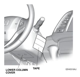
12. Pull away the door opening seal, and remove the driver's dashboard lower cover and unplug the vehicle connectors.
