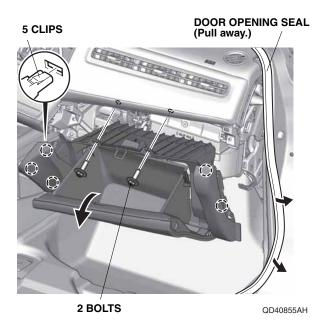
10. Pull away the door opening seal, and remove the driver's dashboard side lid.
