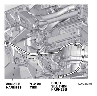
33. Secure the door sill trim harness to the vehicle harness with one wire tie.
