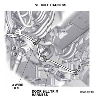
32. Route the door sill trim harness as shown. Secure the door sill trim harness to the vehicle harness with three wire ties.
