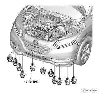
Remove the four clips and two self-tapping screws on each side.
