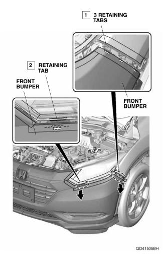
With the help of an assistant, remove the front bumper and unplug the vehicle connectors, if equipped. Place the front bumper on the blanket to prevent damage.
