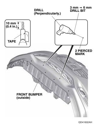
5. While wearing eye protection, drill the four pierced marks to 8 mm.
