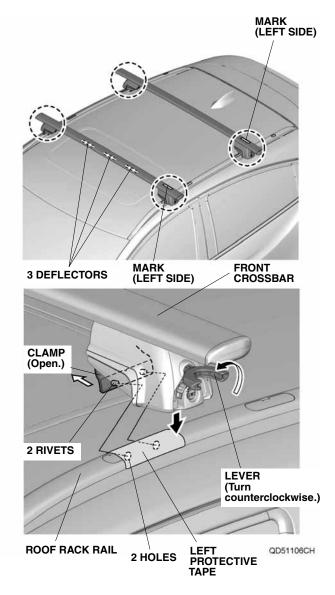
11. Align each rivet with the holes on the roof rack rail, and position the front crossbar. Make sure the crossbar is on the protective tapes.
