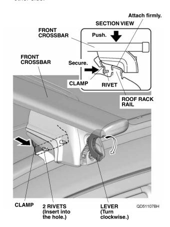
Lower the lever, and lock with key. Repeat on the other side.
