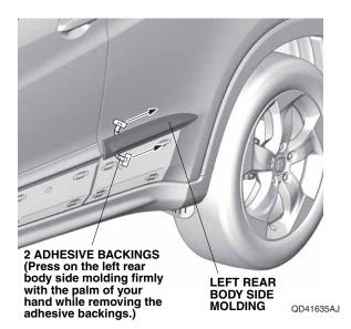
11. Using the rubber roller, apply firm pressure while rolling to set the adhesive. Apply firm pressure especially at the ends.
