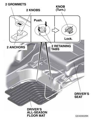
2. Place the grommets in the driver's all-season floor mat over the anchors. Push the grommets into the anchors to secure the retaining tabs, then turn the knobs 90° to secure the all-season floor mat.
